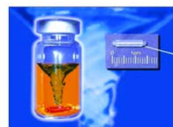
Fig. 1 Stir Bar Sorptive Extraction (SBSE) in Manual do equipamento da Gerstel "Operation Manual Twister Desorption Unit TDU"
